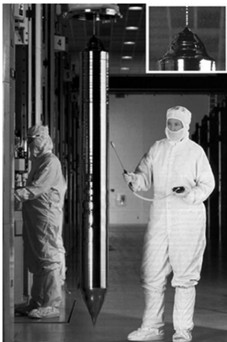
Fig. D.4 200 mm dia., 2 m long, Si single crystal grown by the Czochralski arrangement in a silicon foundry. Single crystals of this size, and even larger, are routinely grown dislocation free, with little macrosegregation of the dopant. Inset on photograph shows the starting seed and the bell-shaped shoulder region which flares out to the final diameter. These crystals are a basic commodity needed by the semiconductor device industry. Adapted from [2]
